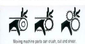
Disconnect and lockout all power before servicing machine. Failure to follow the above can result in severe personal injury.
